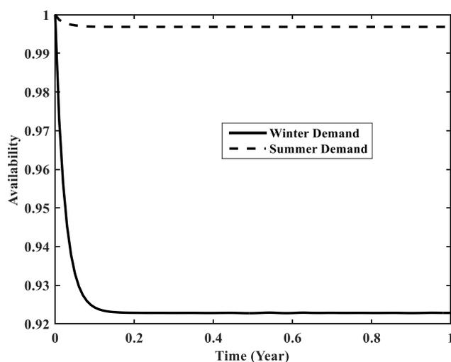
Figure 4. Availability of traction drives in Norilsk-type ship for different constant demand levels
