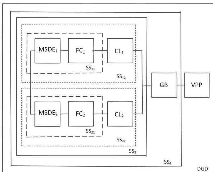
Figure 2. The Reliability Block Diagram of a Norilsk-type ship’s diesel-gear traction drive
