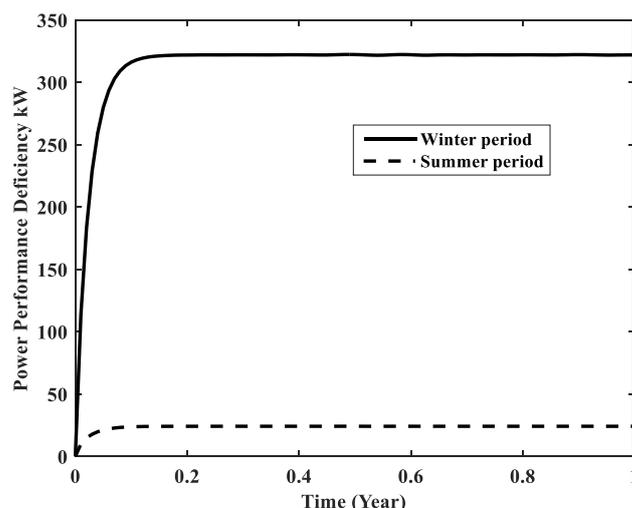
Figure 6. Power performance deficiency of traction drive in Norilsk-type ships
