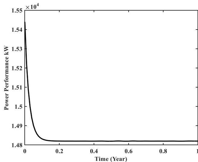
Figure 5. Power performance of traction drive in Norilsk-type ship
