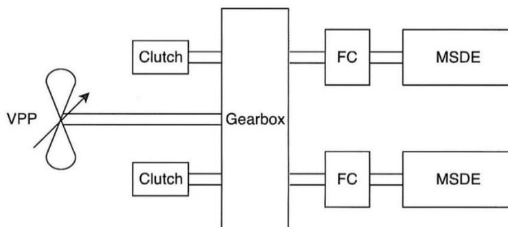
Figure 1. Structure of a Norilsk-type ship’s diesel-gear traction drive
