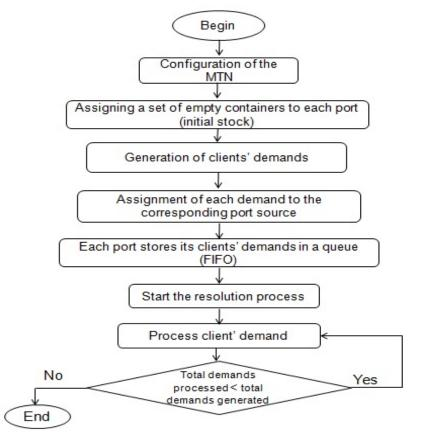
Figure 1. Functional architecture of the proposed application
