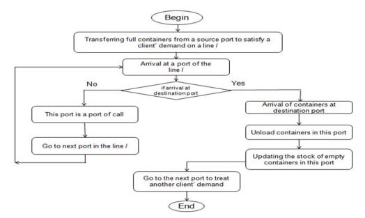
Figure 7. Transfer Process of full containers (source / destination)
