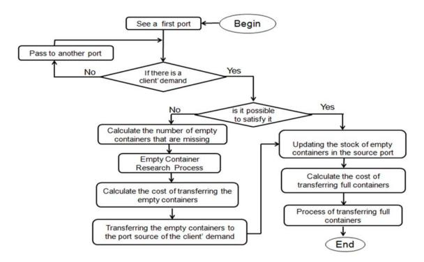
Figure 3. Treatment process of a client demand
