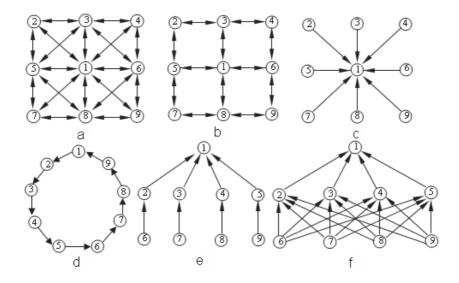
FIGURE 2. Different topologies of PGA [9].
