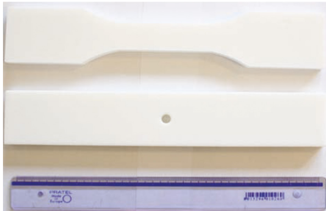
Figure 15. The dumbbell and rectangular prism with hole specimens printed in the SLS technology
