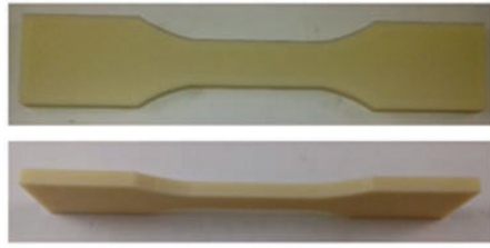
Figure 4. Printed dumbbell specimen (high: 210 mm)
