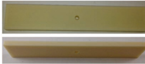
Figure 5. Printed rectangular prism with hole specimen (high: 210 mm)
