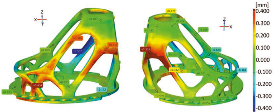
Figure 22. The three-dimensional air turbine head specimen scan with nominal layer thickness 0.028 mm (PolyJet method)
