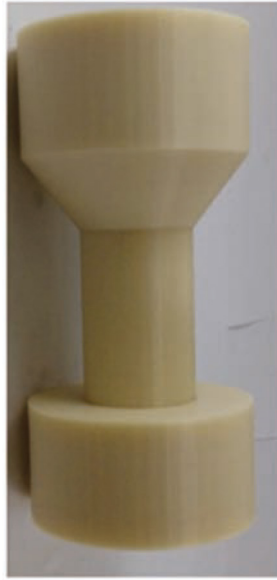
Figure 10. The printed three-dimensional cylinder specimen (high: 160 mm)
