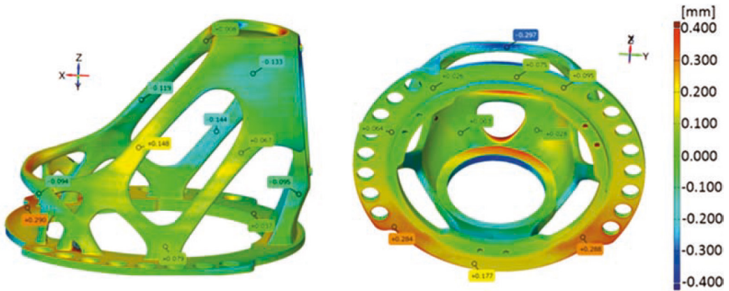
Figure 18. The three-dimensional air turbine head specimen scan with nominal layer thickness 0.120 mm (SLS)
