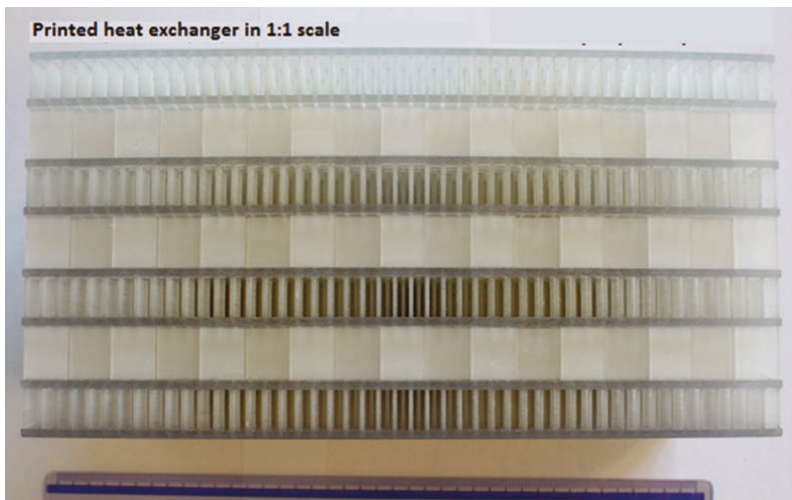
Figure 31. The heat exchanger model printed in 1:1 scale in the PolyJet method (SUP 707 support)
