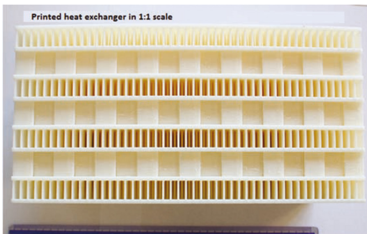
Figure 26. The heat exchanger model printed in 1:1 scale in FDM technology (with support)
