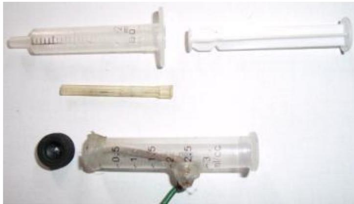
Fig. 5. Potential measuring device in disassembled state.
