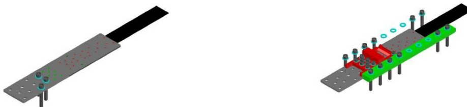
Figure 2: Steel anchorages; passive anchorage mounted on the CFRP strip (left); active anchorage with leading rails and reaction block (right)
