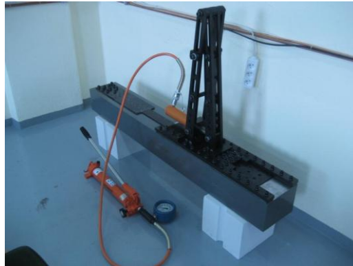
Figure 1: Experimental assembly of NPS system; active anchorage along with the stretching device (right); passive anchorage fixed to the steel beam (left)
