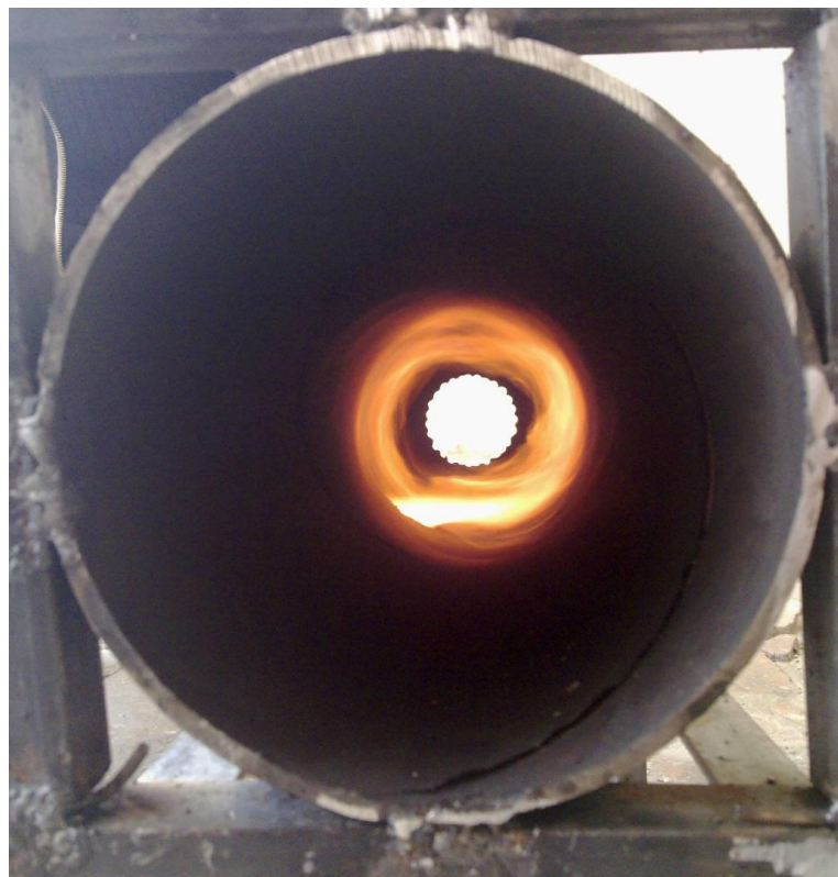
Figure 5: Pilot plant. View from the throttle valve (an axial hole open)
