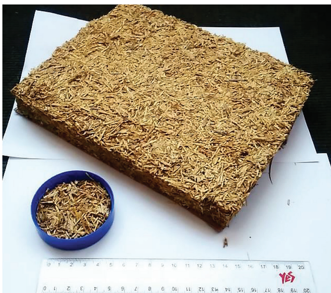
Fig. 2 Flax straw and flax straw lightweight insulation composite
