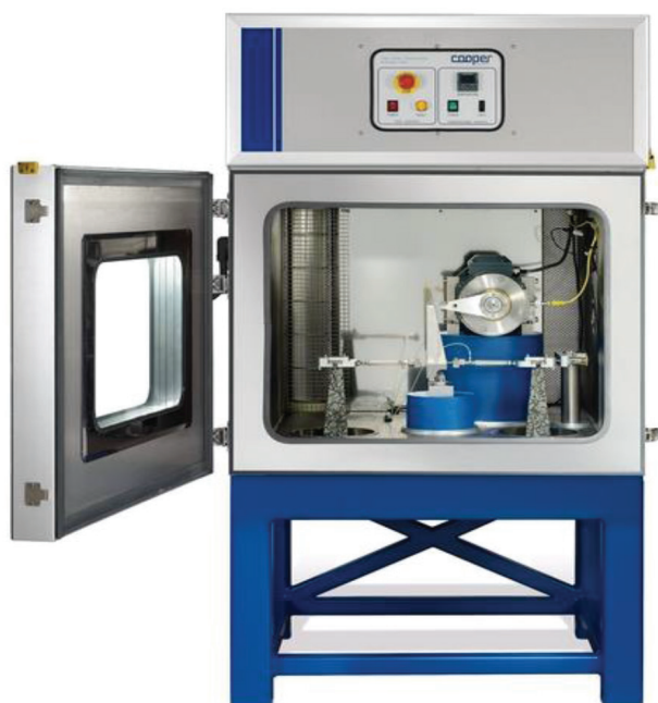
Figure 3: Two-point trapezoidal bending beam machine (Cooper technology, 2017).
