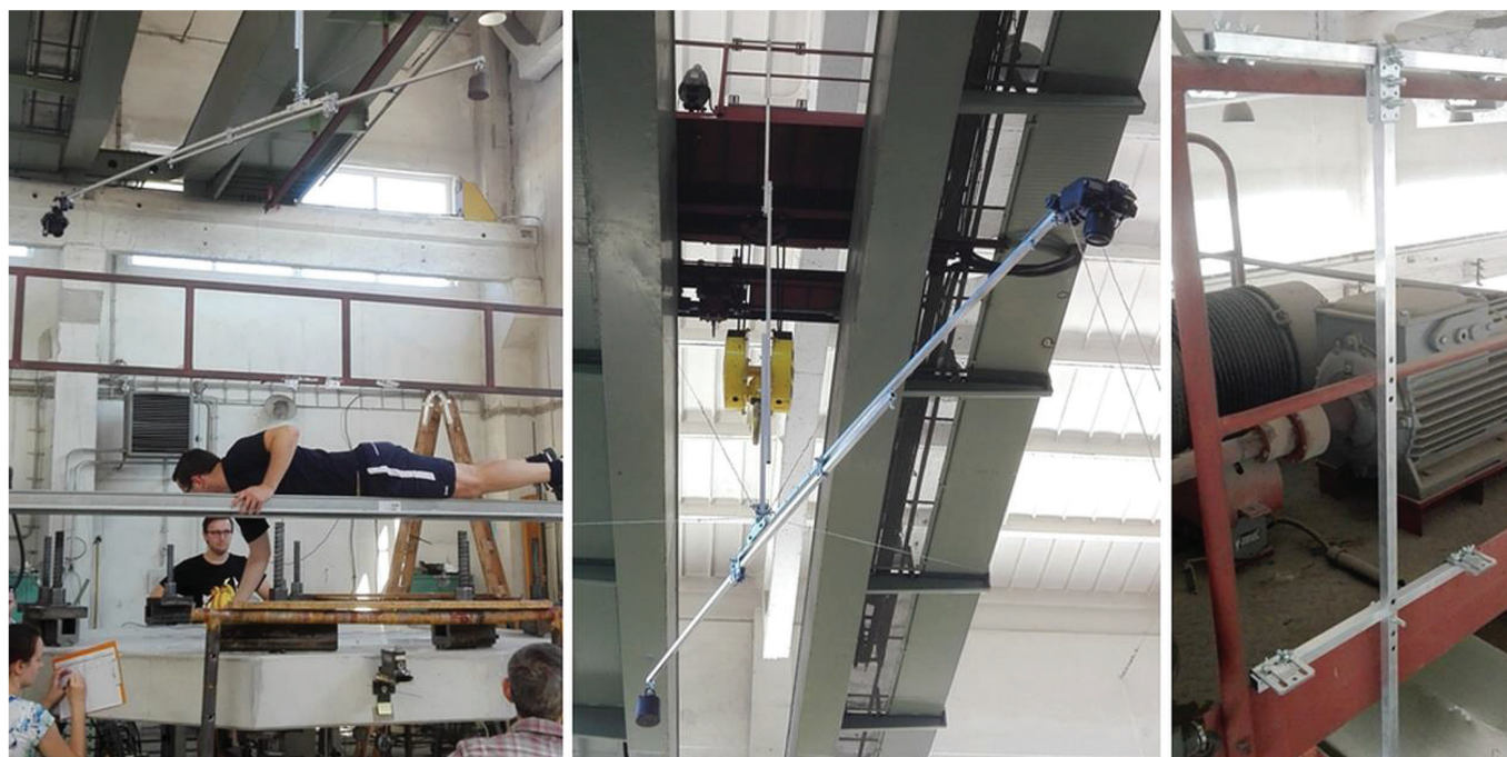
Fig. 2 Hanging mounting construction with camera above the experiment and its stabilisation on a crane.
