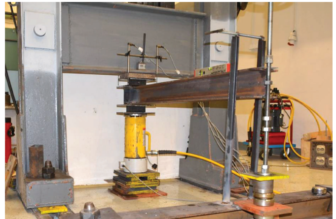
Fig. 11 Testing equipment for the restoring moment test method.
