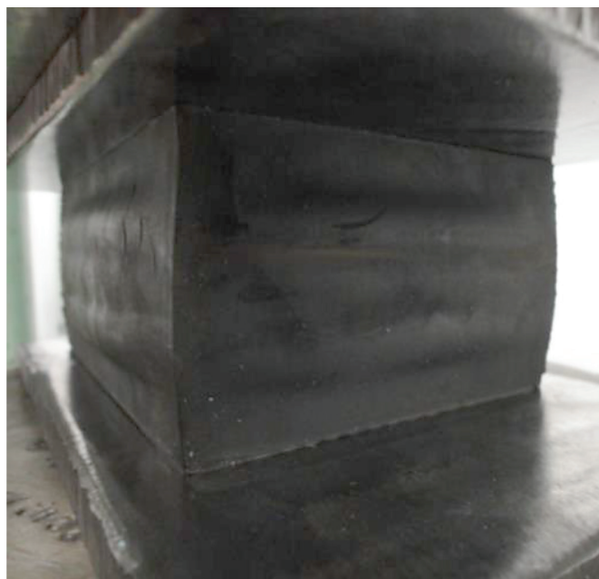
Fig. 15 Bearing under a compressive load.
