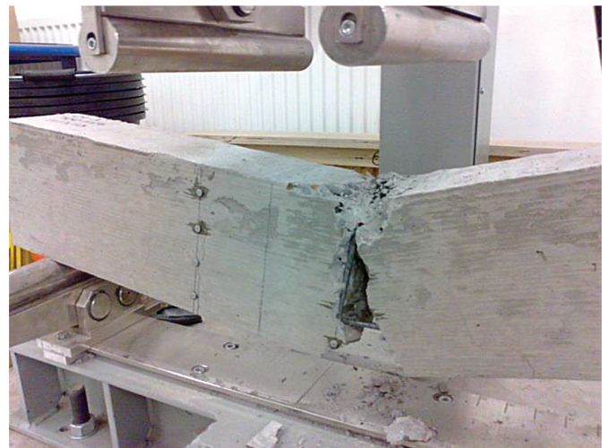
Fig. 16 Failure of the beam containing 100% FEG
