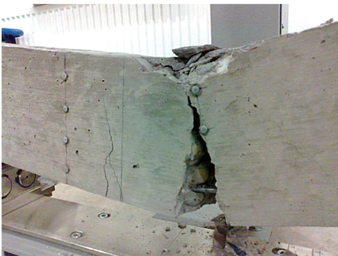
Fig. 14 Failure of the beam containing 25% FEG.
