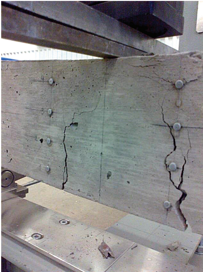
Fig. 13 Failure of the beam containing 0% of FEG.
