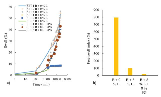
Fig. 3 Variation of (a) the percentage swell over time (b) free swell index for the mixes.
