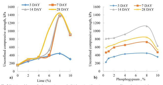
**Fig. 2** *Variations of the unconfined compressive strength of (a) bentonite with varying percentages of lime and curing periods (b) bentonite+8% lime with varying percentages of phosphogypsum and curing periods.*
