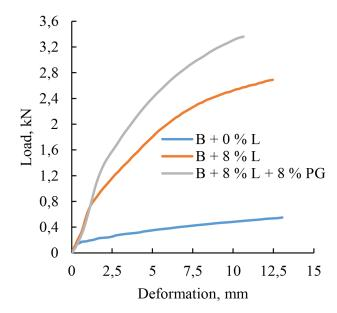
Fig. 7 Load vs. deformation curves obtained in CBR.
