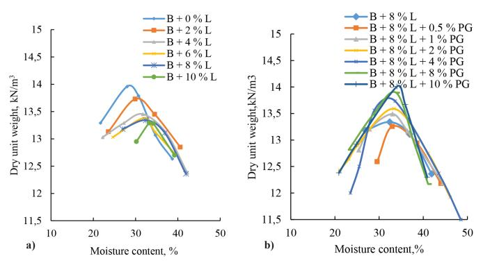
Fig. 1 Compaction curves for (a) bentonite with varying percentages of lime (b) bentonite + 8 % lime with varying percentages of phosphogypsum.
