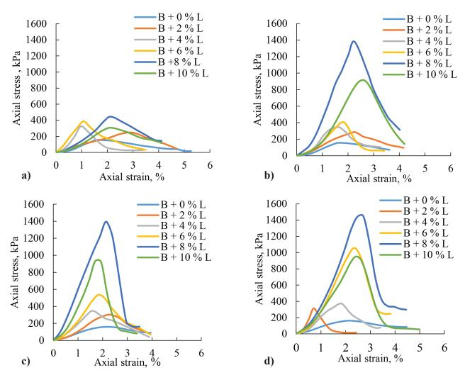
Fig. 5 Variations of axial stress for bentonite mixed with varying percentages of lime at (a) 3 days (b) 7 days (c) 14 days (d) 28 days.
