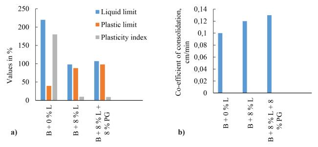
Fig. 4 Variation of the (a) consistency limits (b) coefficient of consolidation for the mixes.
