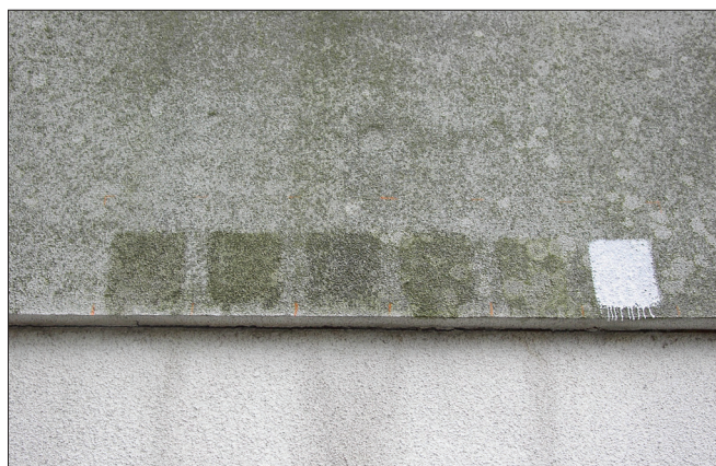
Fig. 1 Records of decontamination experiment on ETICS in 2005. Record created 7 days after the application of six different products. Noted decrease of new microorganisms, e.g., in Squares No. 1 and 2 (from the left) to half the amount (Antošová, N., 2007).
