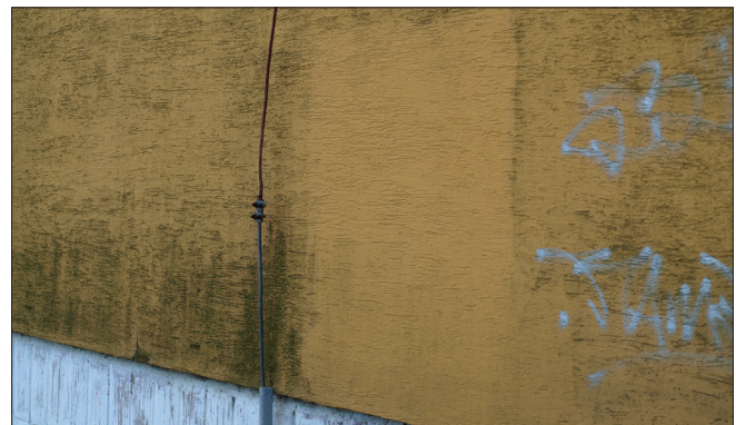
Fig. 7 Records of the decontamination experiment on the ETICS. State of the sample in January 2012; this sample was washed with water after the application of a biocide. (Picture from the archives of the author's experiment)
