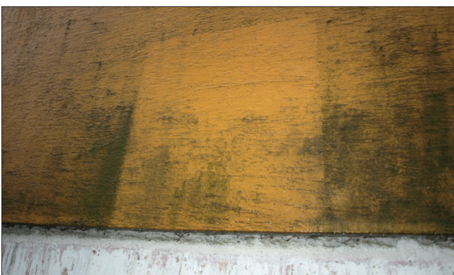
Fig. 8 Records of the decontamination experiment on the ETICS. State of the unwashed sample from Fig. 6, now in January 2013. (Picture from the archives of the author's experiment).
