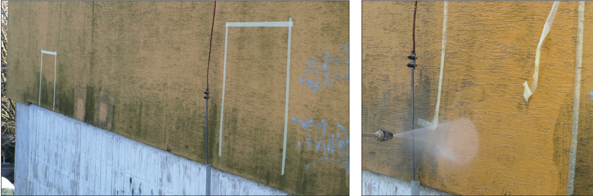
Fig. 5 Records of the decontamination experiment on ETICS in 2011. The state before the application – outlining the area. Cleaning with high-pressure water after 24 hours. (Picture from the archives of the author's experiment).
