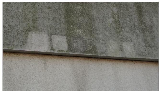
Fig. 4 Records of the decontamination experiment on ETICS in 2009. Note the increase in new microorganisms except in Square No. 1 (from the left). Sample No. 1- destruction of microorganisms outside the designated area (Picture from the archives of the author's experiment).
