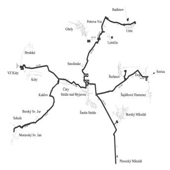
Fig. 1 Scheme of part of the Senica group water supply system.
