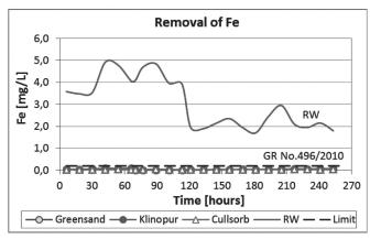
Fig. 5 Course of removing the iron from the water.
