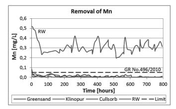
Fig. 8 Course of removing the manganese from water.
