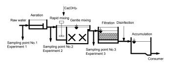
**Fig. 2** Scheme of the technology of WTP Kúty and the location of the filter columns.
