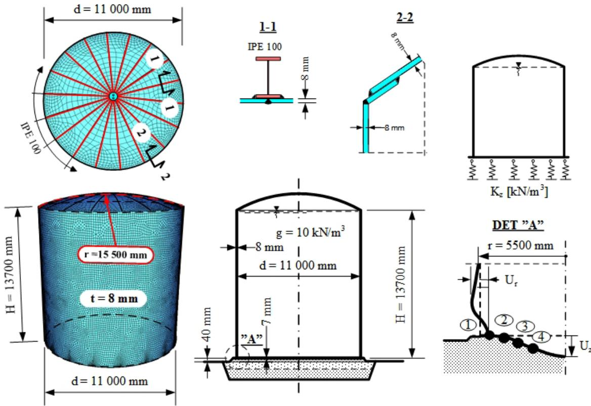
Figure 4: Geometry of the analyzed steel tank on a type A foundation and vertical deformations of the bottom plates  $u_z$  and radial deformations of the cylinder shell  $u_r$ .
