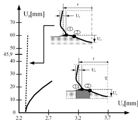
Figure 7: Comparison of vertical deformations  $u_z$  of tank bottom plates and radial deformations  $u_r$  at the point No. 2 for type A and type B foundations of uniform stiffness  $K_z$  (Fig. 4, Fig. 5).
