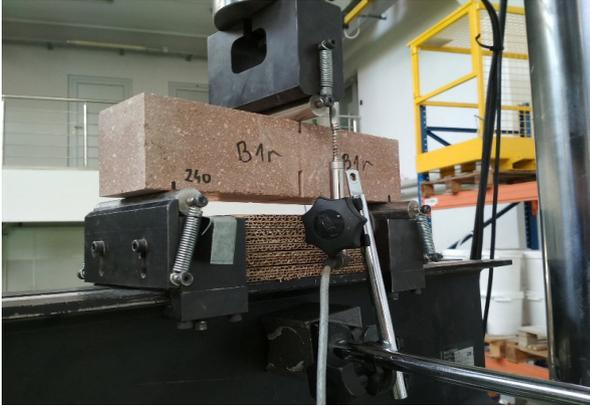
Figure 7: Three point bending test for notched beams.
