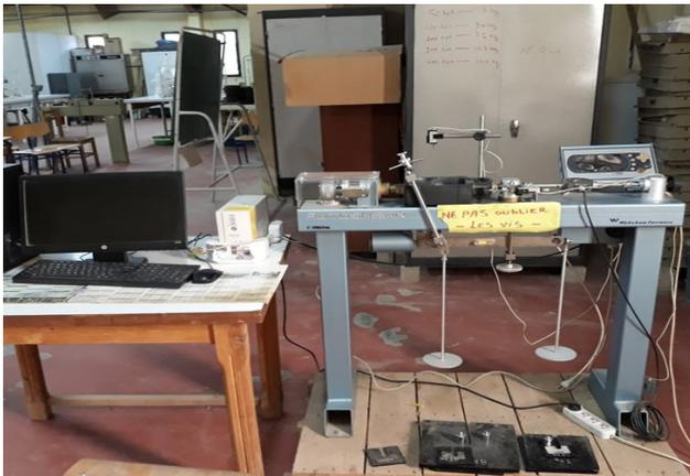
Figure 5: View of the direct shear box apparatus.
