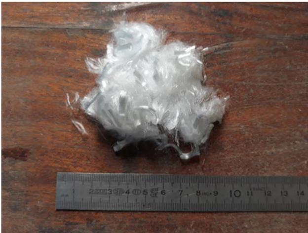
Figure 3: Monofilament polypropylene fiber.
