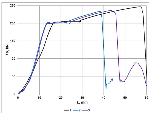
Figure 7: Courses of load as a function of elongation under static load.
