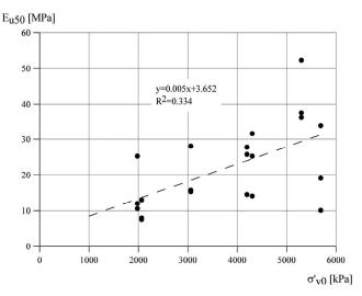
Fig. 3. The undrained modulus  $E_{u50}$  versus effective vertical stress in situ  $\sigma'_{vo}$
