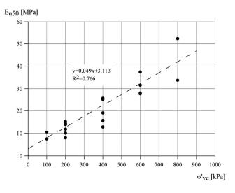
Fig. 4. The undrained modulus  $E_{u50}$  versus effective vertical consolidation stress in situ  $\sigma'_{uv}$
