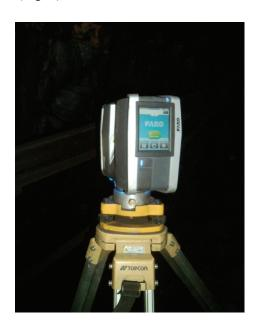
Fig. 3. The FARO Focus 3D scanner during operation
