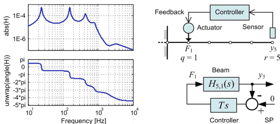
Fig. 6 Frequency response function  $j\omega H_{5,1}(\omega)$  and the AVC system of the cantilever beam
