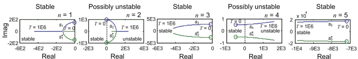
Fig. 7 Root locus to demonstrate the effect of the time constant  $T$  change
