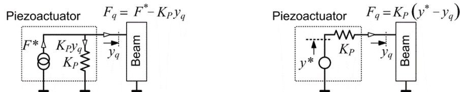
Fig. 5 Two ways of connection of piezo-actuator and beam models
