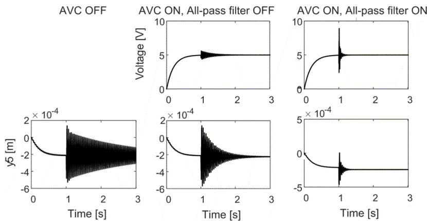
Fig. 10 Decaying vibration without any active control and two ways of the active vibration controls
