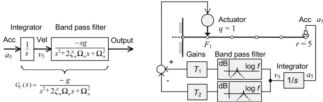
Fig. 8 Principle of Positive Position Feedback (PPF)
