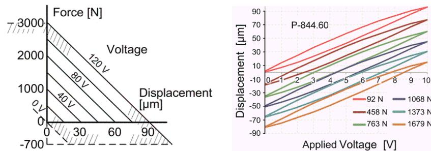
Fig. 3 Working graph for the P-844.60 piezo-actuator and hysteresis measurements
