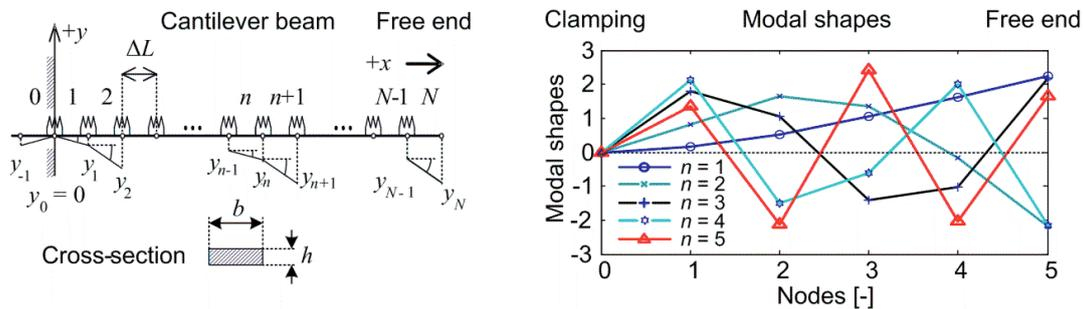
Fig. 1 Coordinates and elements of a cantilever beam, modal shapes
