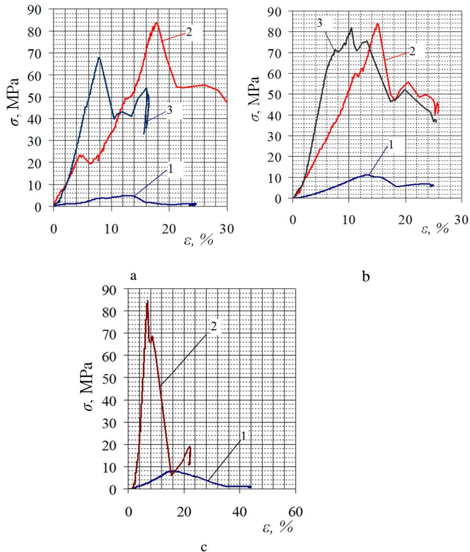
Fig. 9. Stress-strain curves of the bone material of chickens of different ages: a - femoral bone; b - tibia; c-shoulder bone: 1 - 28 days, 2-42 days, 3-49 days
