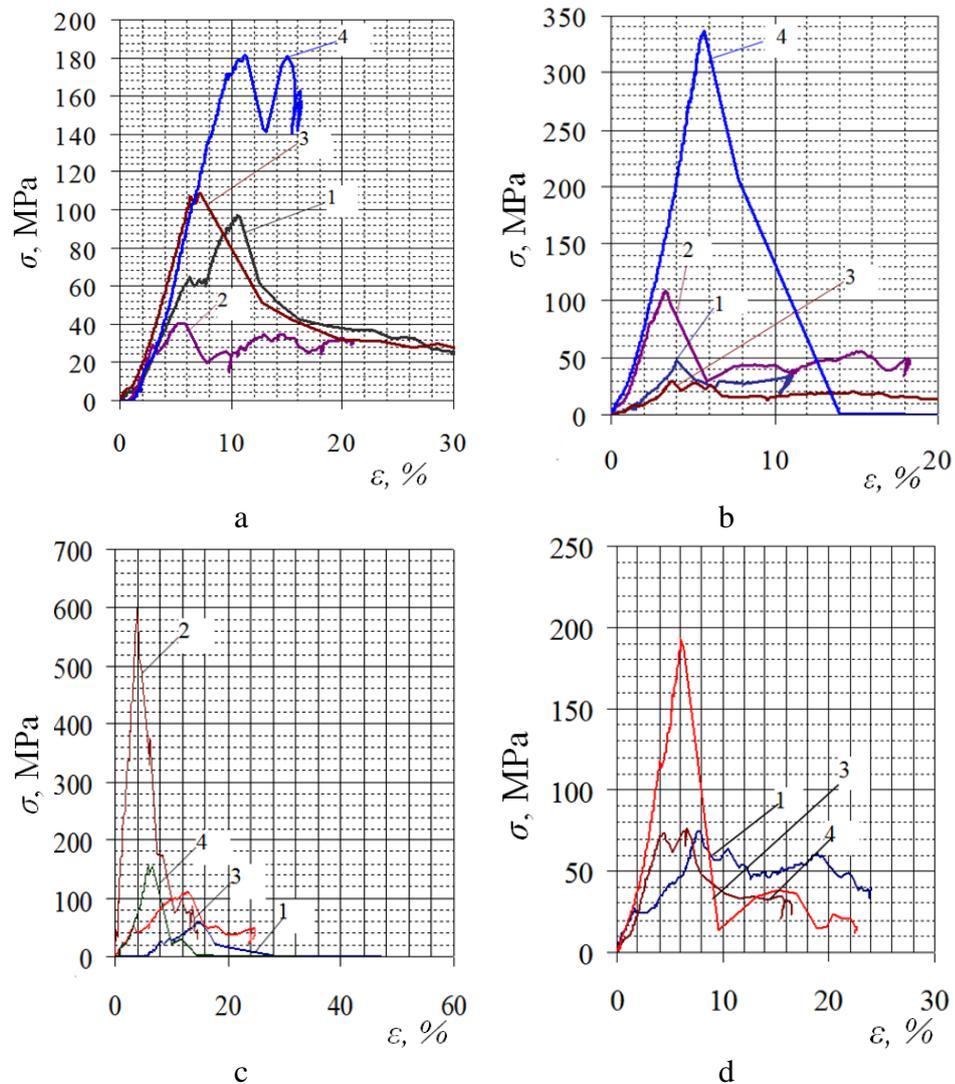
Fig. 5: Stress-strain curves of bone material of chickens of different ages: a - femoral bone; b - tibia; c - elbow bone; d - shoulder bone; 1 to 51 days, 2 to 114 days, 3 to 175 days, 4 to 410 days
