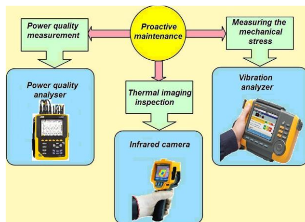
Figure 1. The main components of predictive maintenance in the electrical engineering [11, 12].
