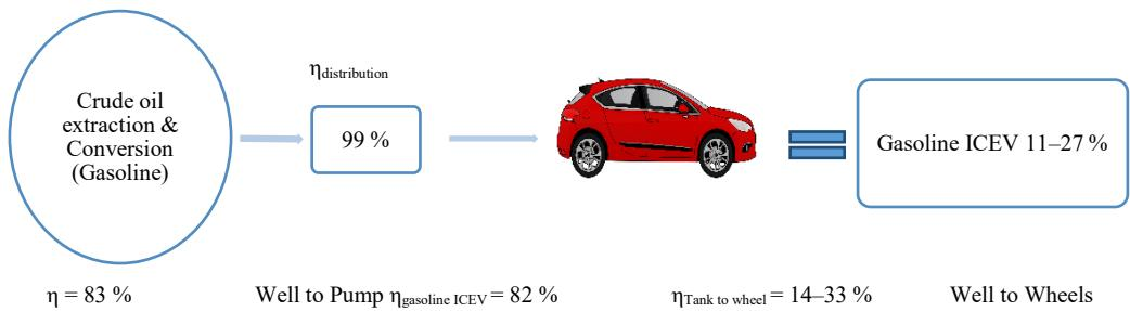
Fig. 1. WTW efficiency of gasoline ICEV.
