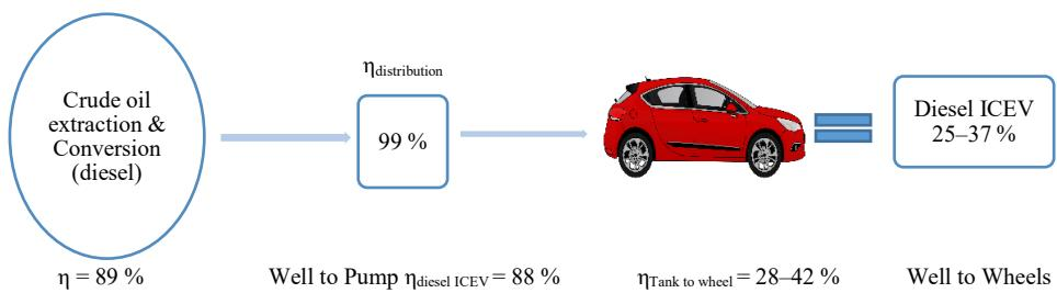
Fig. 2. WTW efficiency of diesel ICEV.
