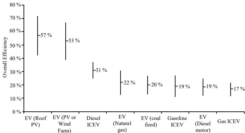
Fig. 6. Overall efficiencies for different cars powered from different sources.
