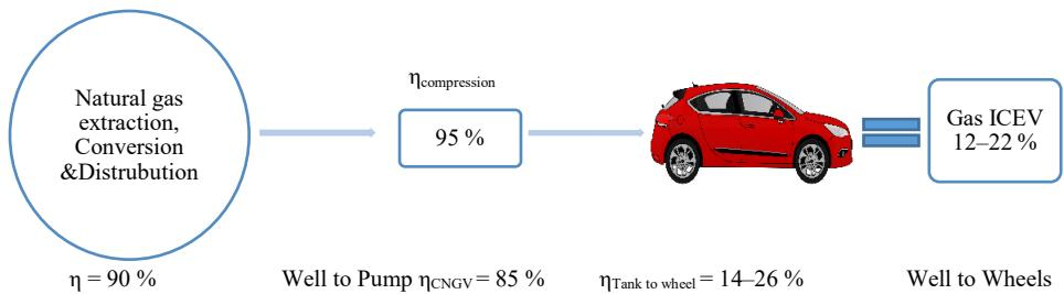
Fig. 3. WTW efficiency of CNGV.
