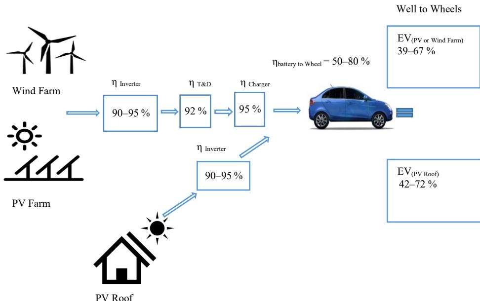
Fig. 5. WTW efficiency of EVs from renewable energy sources.
