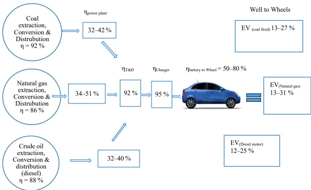
Fig. 4. WTW efficiency of EVs powered from fossil fuels power plants.
