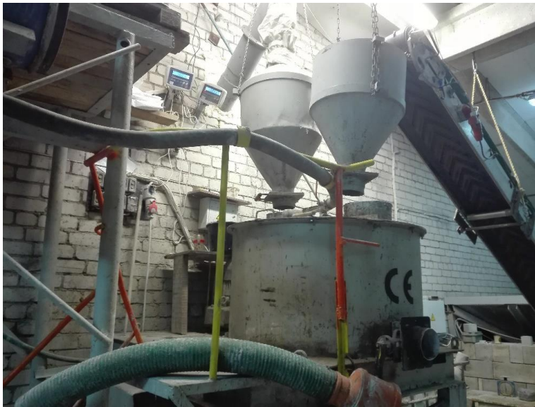
Fig. 1. Turbulence mixer with cavitation effect in the foam concrete plant (intensive mixing technology).
