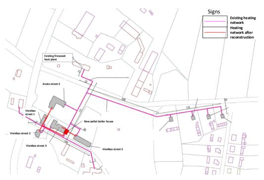
Fig. 1. Analysed DH network before and after reconstruction [35].
