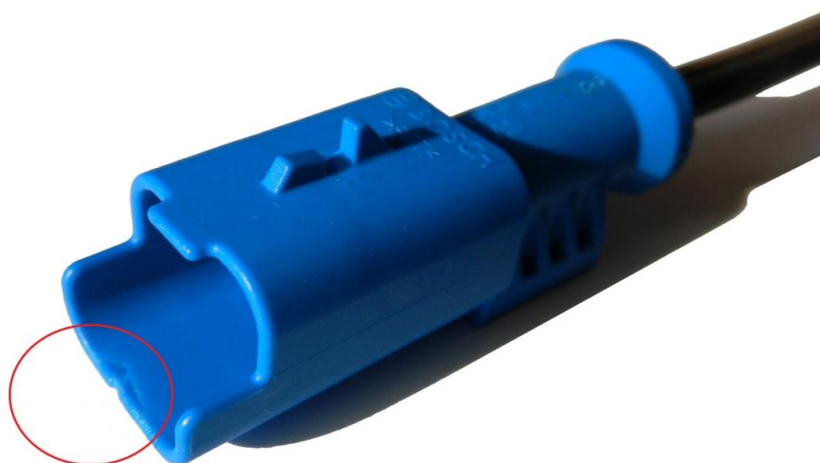
Fig. 1 The reject with material degradation caused by diesel effect
