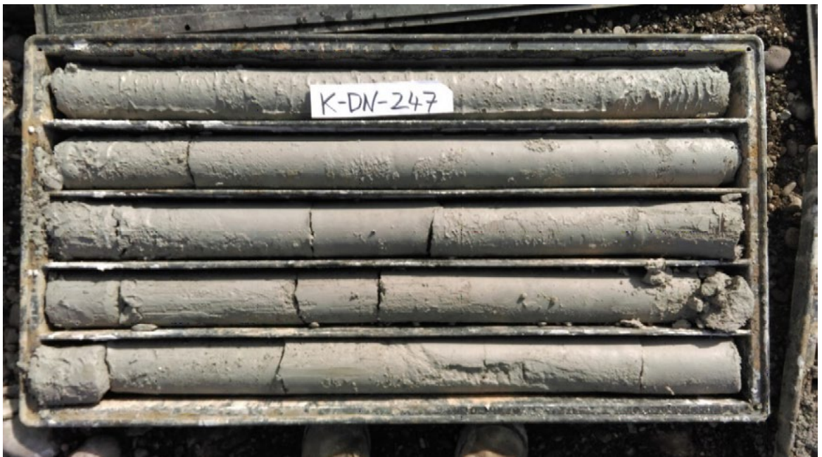
Figure 6. Core obtained through the use of high-frequency core drilling (source: Gecko Ltd.).
