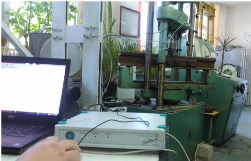
**Figure 4.** General view of the set-up of the rail joint testing.
