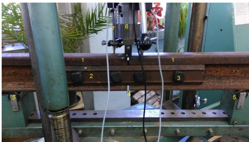
**Figure 5.** Main components of the set-up of the rail joint testing: 1. rail end; 2. joint bar; 3. bolt; 4. joint gap; 5. support; 6. piercer; 7. displacement transducer.
