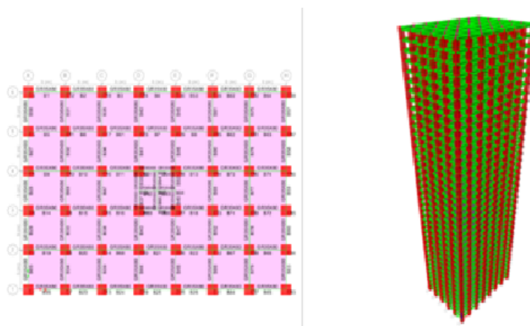
Figure 11. Reinforced concrete framed structure with a rectangular shape 40 levels – plane and elevation
