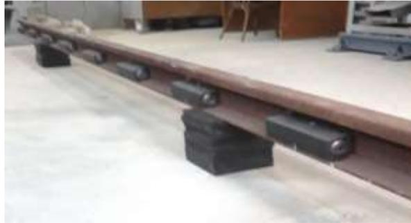
**Figure 6.** Rail coupon with dampers on resilient supports.
