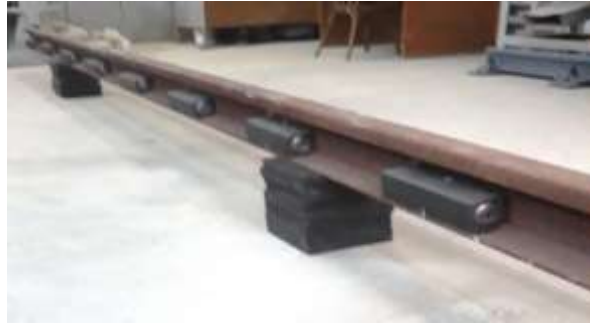
Figure 6. Rail coupon with dampers on resilient supports.
