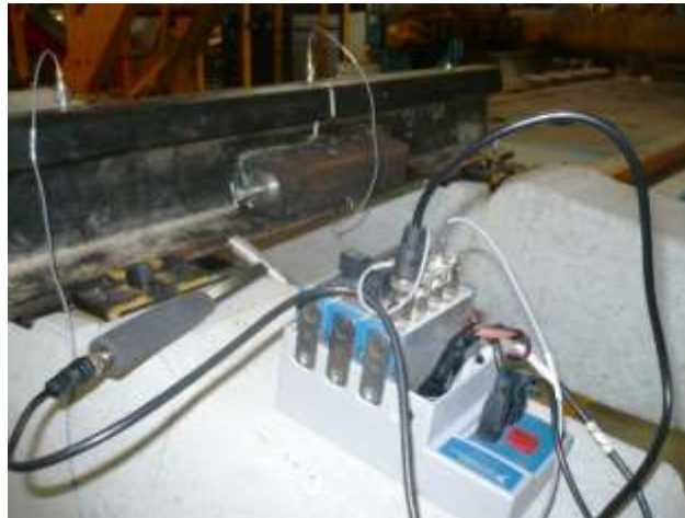
Figure 3. Set-up of the testing of the rail damper functionality
