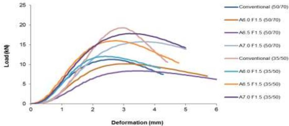
**Figure 8.** Load-deformation curves for asphalt mixtures subjected to water conditioning
