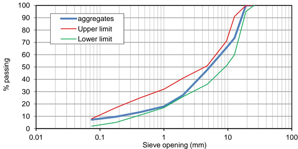
**Figure 1.** Aggregate gradation used for the asphalt mixtures
