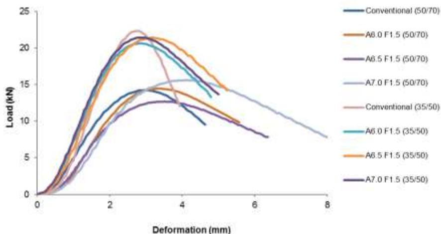
**Figure 7.** Load-deformation curves for asphalt mixtures subjected to air conditioning
