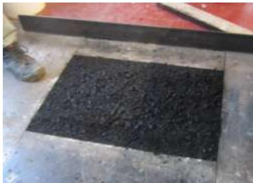
**Figure 3.** Asphalt mixture compacted in a slab mold using a steel roller compactor
