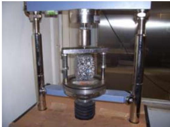
**Figure 5.** Indirect tensile strength test apparatus
