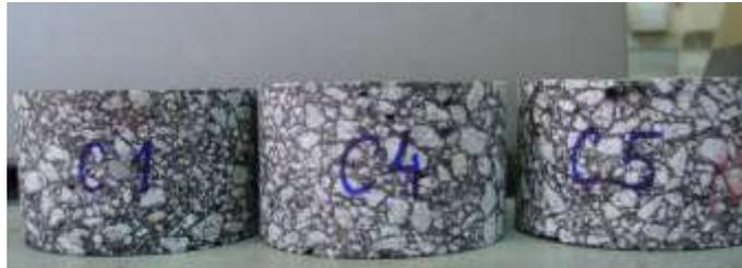
**Figure 4.** Cylindrical specimens used in the indirect tensile strength tests
