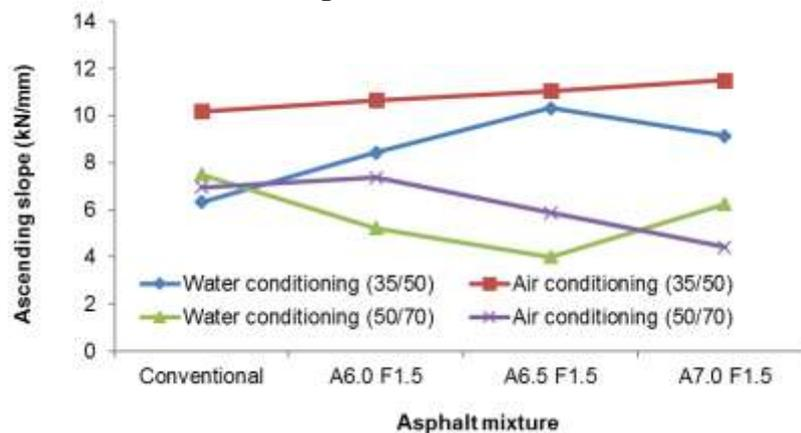
**Figure 11.** Ascending slopes of the load-deformation curve
