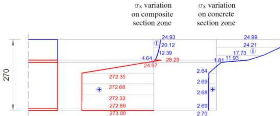
**Figure 16.**  $\sigma_x$  variation on the section height in the two materials (steel and concrete)
