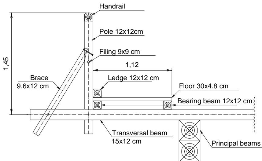
Figure 1. Sidewalk structure
