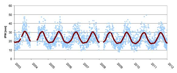
Fig. 20. IPW for PDEL (Azores) and model with 3 oscillations (annual and 1/2, 1/3 -year) applied to 2003-2012 period
