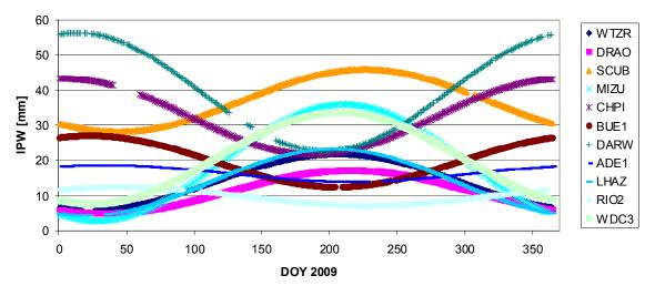
Fig. 4. Integrated precipitable water annual model for selected IGS stations in 2009 (CODE global solution)
