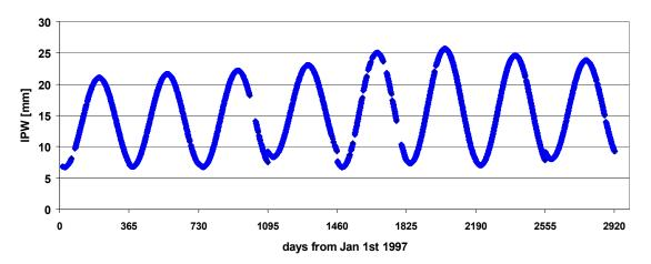
**Fig. 9.** Results for 8 years (1997-2004) for JOZE from IGS CODE global solution, during first 5 years period there is +0.6 mm/year IPW trend. For the following years not visible. Each year is fitted separately – so the jumps at the year beginning.
