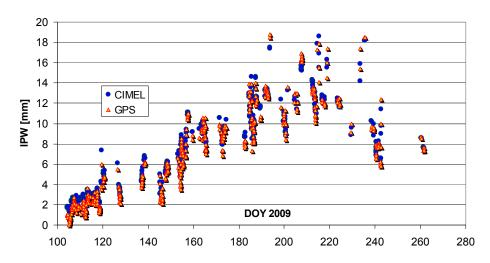
**Fig. 10.** Hornsund IPW from CIMEL-318 measurements and GPS in 2009 (only hours with both measurements available)
