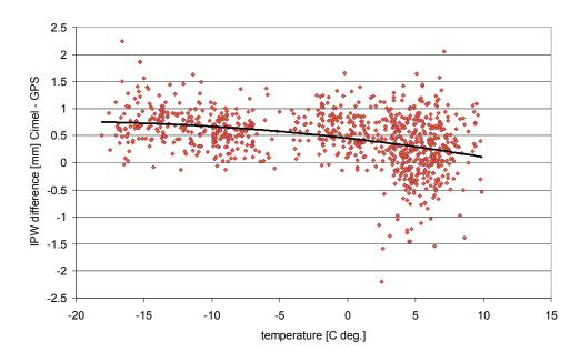
**Fig. 15.** IPW difference (CIMEL-318 - GPS) for Hornsund in 2008-2010 wrt. surface atmospheric temperature
