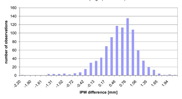
**Fig. 13.** IPW difference histogram at Hornsund (CIMEL-318 measurements minus GPS) for the whole campaign (2008-2010)
