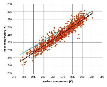
**Fig. 2.** Mean temperature vs. surface temperature for Ny Alesund, 2008-2010 (1134 soundings), linear formula fitting (black line) and Bevis formula (blue line)
