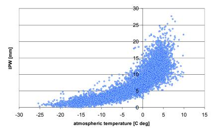
**Fig. 4.** Hornsund IPW vs. atmospheric temperature - the whole campaign (original 3 hour interval of meteorological measurements)
