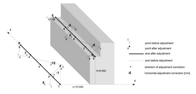
**Fig. 2c.** Horizontal adjustment corrections in the *xyz* system
