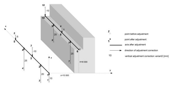
Fig. 2b. Vertical adjustment corrections in the *xyz* system [variant 2]
