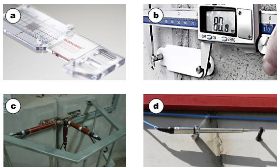
**Figure 1.** Different measurement solutions: (a) simple ‘crackmeter’ (source: [www.avongard.com](http://www.avongard.com)), (b) measurement solution of SHM-X company (source: [www.shmsystem.pl](http://www.shmsystem.pl)), (c) electronic extensometers in a 3D measurement system and (d) SisGeo linear extensometer (source: [www.sisgeo.com](http://www.sisgeo.com)).
