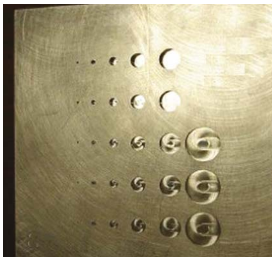
FIGURE 1. Structure of the PTW EPID QC PHANTOM®, 1. Signal linearity and signal noise ratio, 2. Isotropy of signal linearity, 3. Geometric isotropy (distortion), 4. Low-contrast resolution, 5. High-contrast resolution (MTF).
