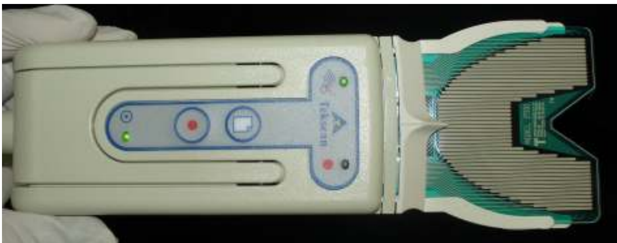
Figure 1 – T-Scan III handler connected directly through USB to the computer and sensor-100 microns thickness
