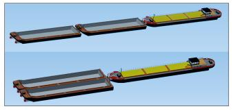
Fig. 4. Convoy of BM-500 and 2 BP-500 barges: up-river configurations (upper drawing) and down-river configurations (bottom drawing)
