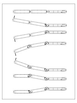
Fig. 8. Turning performance of convoy: BM-500 and 2 BP-500, turning control by bow steering system and dynamic couplings between barges
