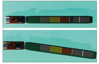
Fig. 7. Turning performance of convoy: BM-500 and BP-500, turning control by bow steering system and dynamic coupling
