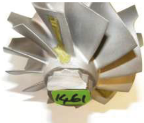
Turbine blade with strain gauge
