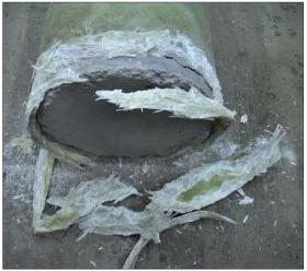
*Fig. 2. Destruction (debonding) of a pipe made of glass fibre reinforced composite*
