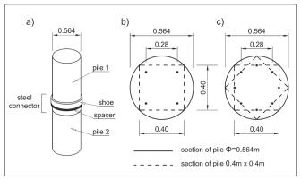
Fig. 15. Steel joint for circular piles in a composite coating: a) diagram for joining piles, arrangement of bolts and sleeves: b) two bolts and two sleeves,
