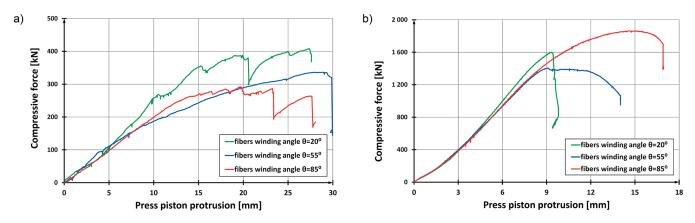
Fig. 10. Relation between force and displacement for: a) coating, b) composite pipe filled with concrete
