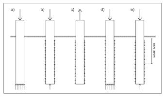
Fig. 4. Scheme of transferring loads through a vertical pile to the soil
