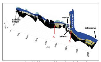
Fig. 2. Numerical model of the section of the Dead Vistula from Sobieszewo Bridge up to its outlet to the Bay of Gdansk together with the branch from the Watershed (Przełom) up to Siennicki Bridge  $(Z_p,Z_2-planned\ sewage\ discharge\ localization\ sites)$
