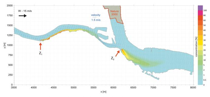
Fig. 6. Calculation results of spreading the pollution in the conditions of the westerly wind W – 15 m/s (Variant 3)
