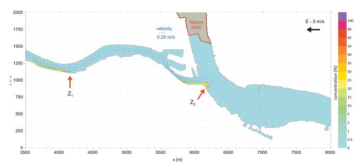
Fig. 4. Calculation results of spreading the pollution in the conditions of the easterly wind  $E-5\ m/s$  (Variant 1)
