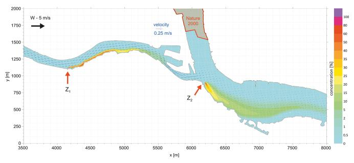
Fig. 5. Calculation results of spreading the pollution in the conditions of the westerly wind W - 5 m/s (Variant 2)
