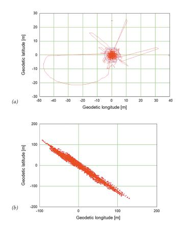
Fig. 3. A position distribution around the mean value for the DGPS system;
