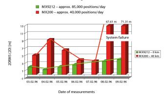
Fig. 2. Position error (determined every 24 h) for two DGPS receivers operating in parallel. Corrections were obtained from the DGPS station in Rozewie [10]
