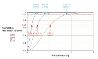
Fig. 4. The cumulative distribution functions of the 2D position errors for the DGPS-PL system (Rozewie) determined in 2006, 2009, 2014 based on 1–2 million measurements per campaign
