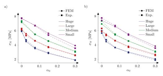
Fig. 6. Nominal (XFEM calculations) and experimental strengths with the bilinear softening curve,  $f_t$ =5.0 MPa and  $G_j$ =48 N/m (a) and the exponential softening,  $f_t$ =4.8 MPa and  $G_t$ =35 N/m (b)
