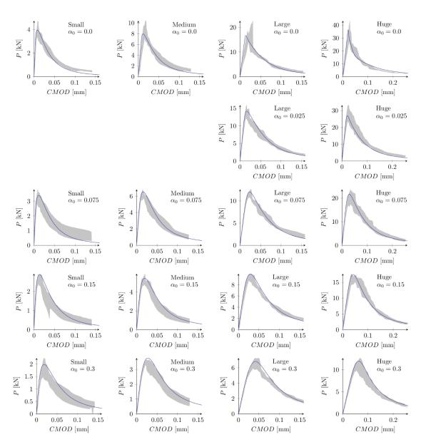
Fig. 10. Experimental and numerical (elasto-plasticity calculations) force – crack mouth opening displacement (CMOD) curves for exponential softening,  $f_i$ =4.8 MPa and  $G_i$ =35 N/m
