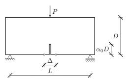
Fig. 3. Boundary conditions and geometry of a beam
