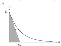
Fig. 2. Bilinear (a) and exponential (b) softening curves (grey area – initial fracture energy)
