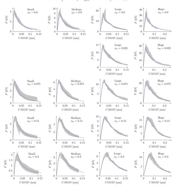
Fig. 7. Experimental and numerical (XFEM calculations) force – crack mouth opening displacement (CMOD) curves for bilinear softening,  $f_i$ =5.0 MPa and  $G_i$ =48 N/m
