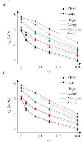
Fig. 9. Nominal (elasto-plasticity calculations) and experimental strengths with the exponential softening curve,  $f_i$ =4.8 MPa,  $G_i$ =35 N/m and the characteristic length l=5 mm (a) and l=2 mm (b)
