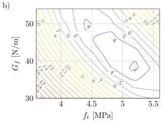
Fig. 5. Error contour maps for seed calculations with XFEM: Err<sub>1</sub> (a) and Err<sub>2</sub> b) (in percentages)
