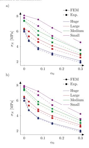
Fig. 8. Nominal (elasto-plasticity calculations) and experimental strengths with the bilinear softening curve, f<sub>=</sub>5.0 MPa, G<sub>=</sub>48 N/m and the characteristic length l=5 mm (a) and l=2 mm (b)
