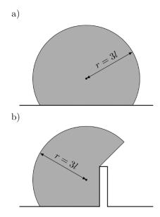
Fig. 1. Averaging domain (grey area) for a point near boundary (a) and close to a notch (b)
