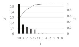
Fig. 4. Pareto-Lorentz diagram which takes into account relations between parameters  $p_{,i}$  their relative values of control quality index  $J_{,i}$  as well cumulated values  $S_{,i}$  determined for  $\eta_{,i} = (5,10,10)$
