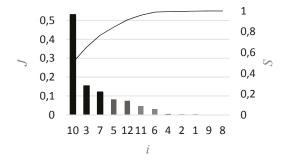
Fig. 2 Pareto-Lorentz diagram which takes into account relations between parameters, their relative values of control quality index J as well cumulated values S, determined for  $\eta_d = (10,10,10)$
