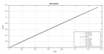
Fig. 7. The desired and real trajectory of the ship for  $\eta_d = (10,10,10)$  and  $\pm 20\%$  change in averaged values of the parameters classified to the groups A, B, C, respectively
