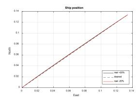
Fig. 3 Diagram of the desired ship's trajectory and real ones for the case:  $\eta_d = (10,10,10)$  with taking into account  $\pm 20\%$  change in values of the parameters of the group A
